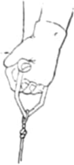
The correctly gripped hammer
